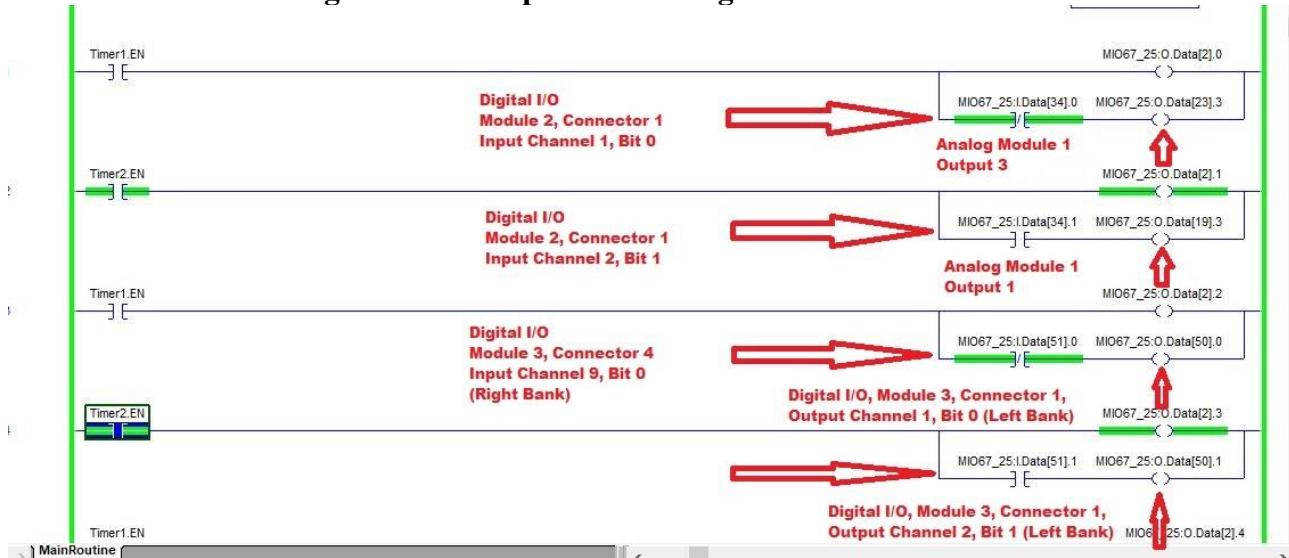
Figure 61 Example Ladder Logic With Modules
